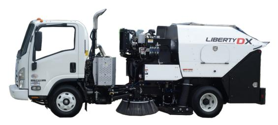
3.32 Cubic Meters High Dump Stainless Steel Debris Hopper
