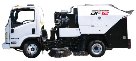
Dual Fuel Sweeper (gas chassis - diesel sweeper)
