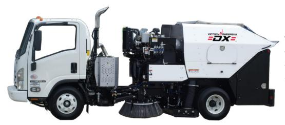
4.35 yd3 High Dump Isuzu NPR HD Diesel 14,500 lbs GVWR 132 inch Wheelbase
