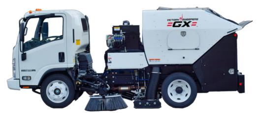
4.35 yd³ High Dump Stainless Steel Hopper Isuzu NPR HD Gas 14,500 LB GVWR 109" Wheelbase
