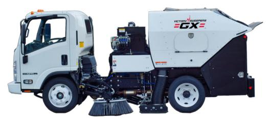
4.35 yd³ High Dump Aluminum Hopper Isuzu NPR Gas 12,000 LB GVWR 109" Wheelbase
