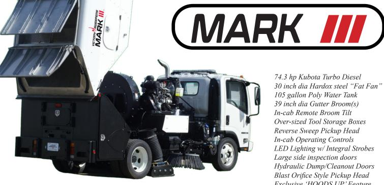
74.3 hp Kubota Turbo Diesel 30 inch dia Hardox steel "Fat Fan" 105 gallon Poly Water Tank 39 inch dia Gutter Broom(s) In-cab Remote Broom Tilt Over-sized Tool Storage Boxes Reverse Sweep Pickup Head In-cab Operating Controls LED Lighting w/ Integral Strobes Large side inspection doors Hydraulic Dump/Cleanout Doors Blast Orifice Style Pickup Head Exclusive 'HOODS UP' Feature
